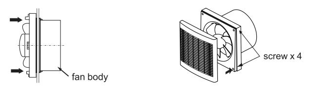
**Step 4:**Centralise the fan body into the hole in the glass.
