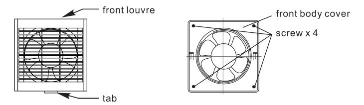
**Step 2:**To open the louvre, pull the bottom tab forward.
